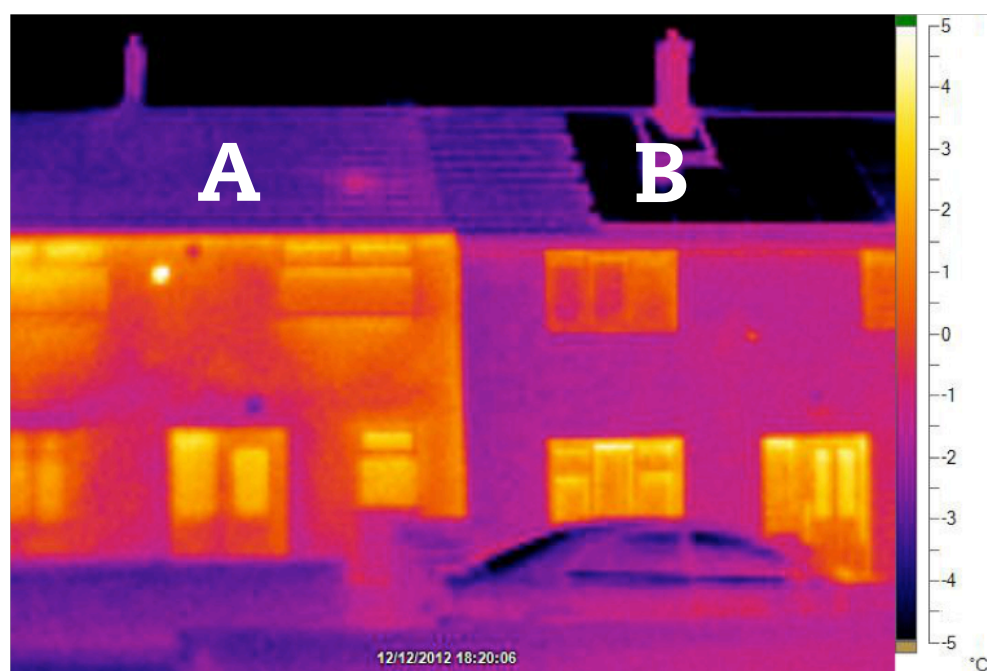
Figure 26: Two Wimpey No Fines properties, (A) has had no insulation works, (B) has had external cladding
