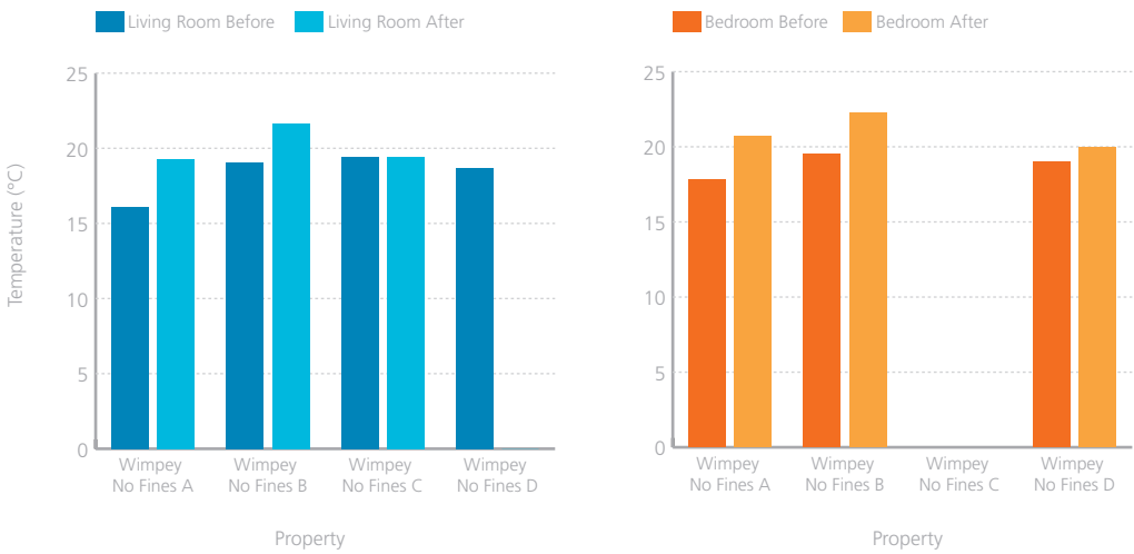
Figure 29: Mean of internal temperatures before and after the works when external temperatures are between -1 and 1°C – Tarran Newlands
